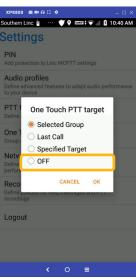
To turn One Touch PTT off, touch "OFF," The radio button will turn orange. When this feature is OFF. pressing the PTT call button will not initiate a call when the screen is off or device is locked.
